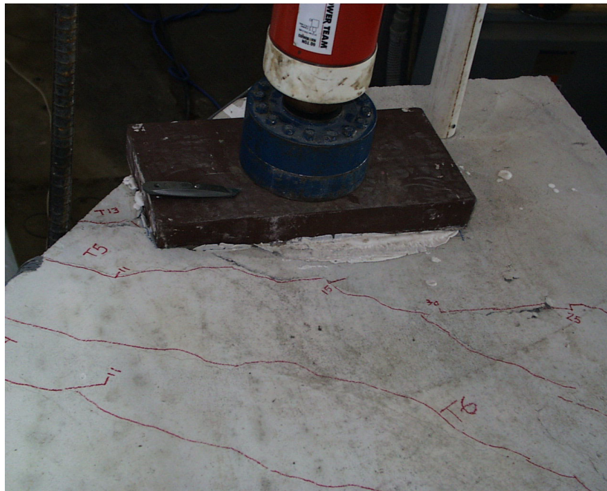
Figure 6-18 Failure of breakback UTSE overhang, top view of slab, facing north
