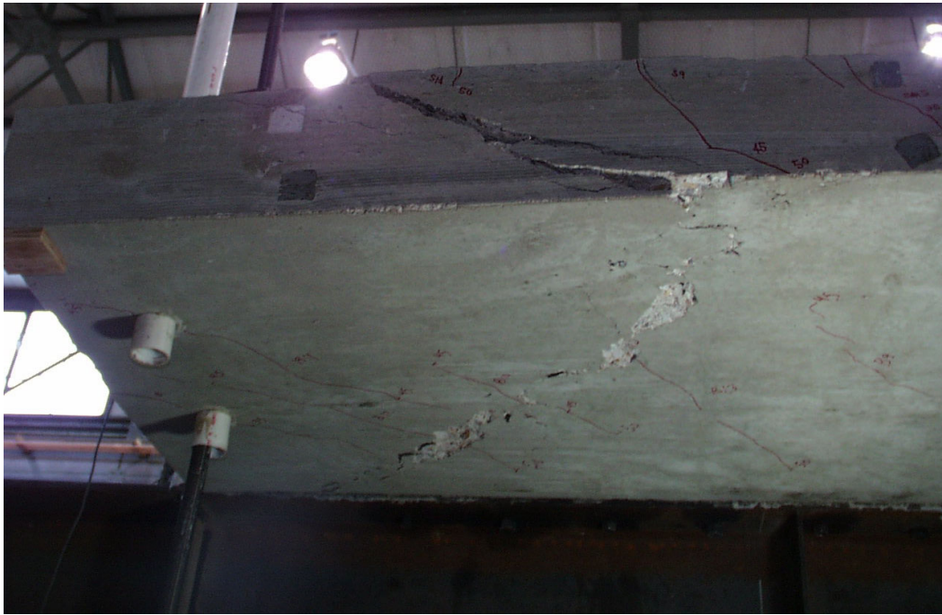
Figure 6-36 Failure of simulated 0° skew UTSE overhang, bottom view of slab, facing east
