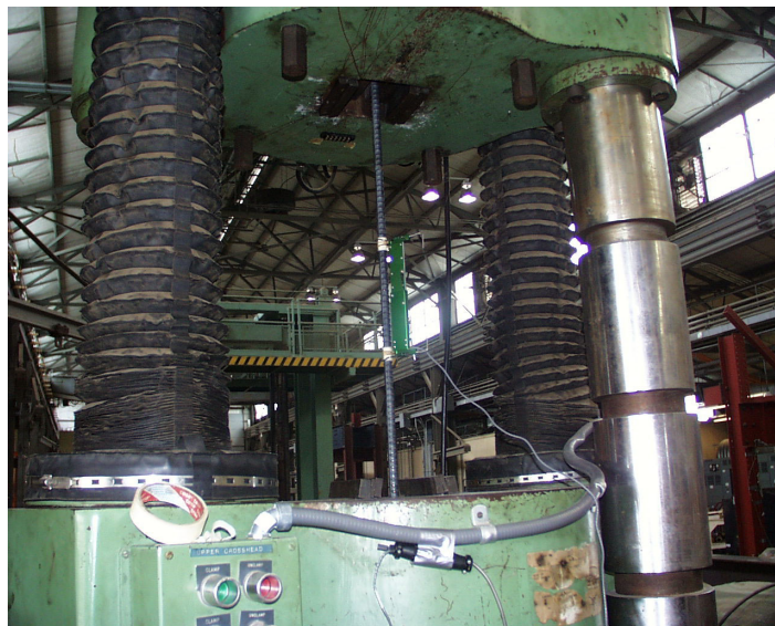
Figure 4-11 Rebar tension test setup 31
